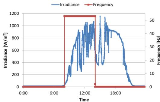
**Figure 7:** Irradiance and frequency of the master pump in a cloudy day.
