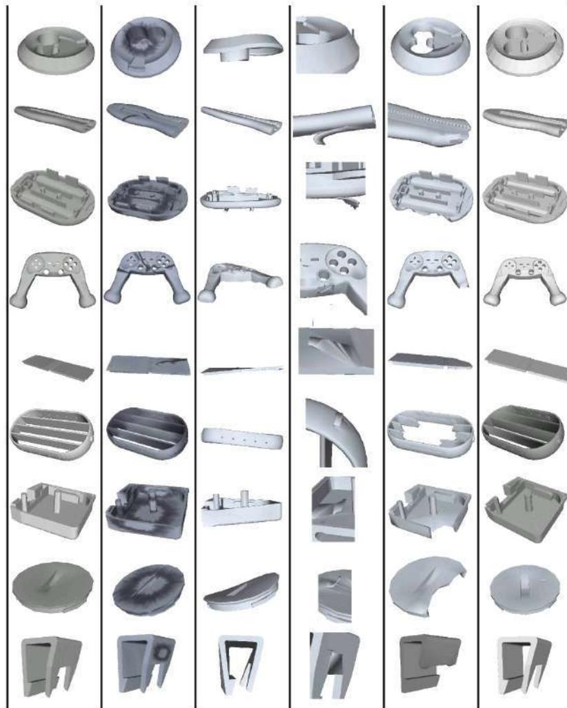
Figure 5.- Examples of visualization of defects occurrence, Burning marks, Warpage, Exfoliation, Short Shots, Ejectors marks
