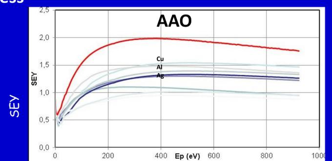
**SEY (Secondary Electron Yield):** The dependence of the SEY on the incident electron energy and impact position of the primary electrons
