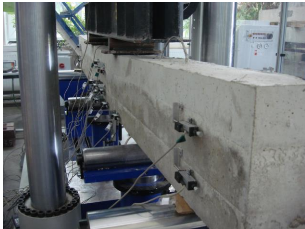
Fig. 1: Multilayered beam (SFRC in external layers and RC in the internal one) during the flexural essay.
