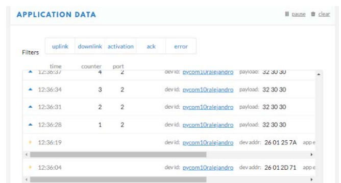
Figure 10: Screenshot of the data sent from the device to the TheThingsNetwork platform
