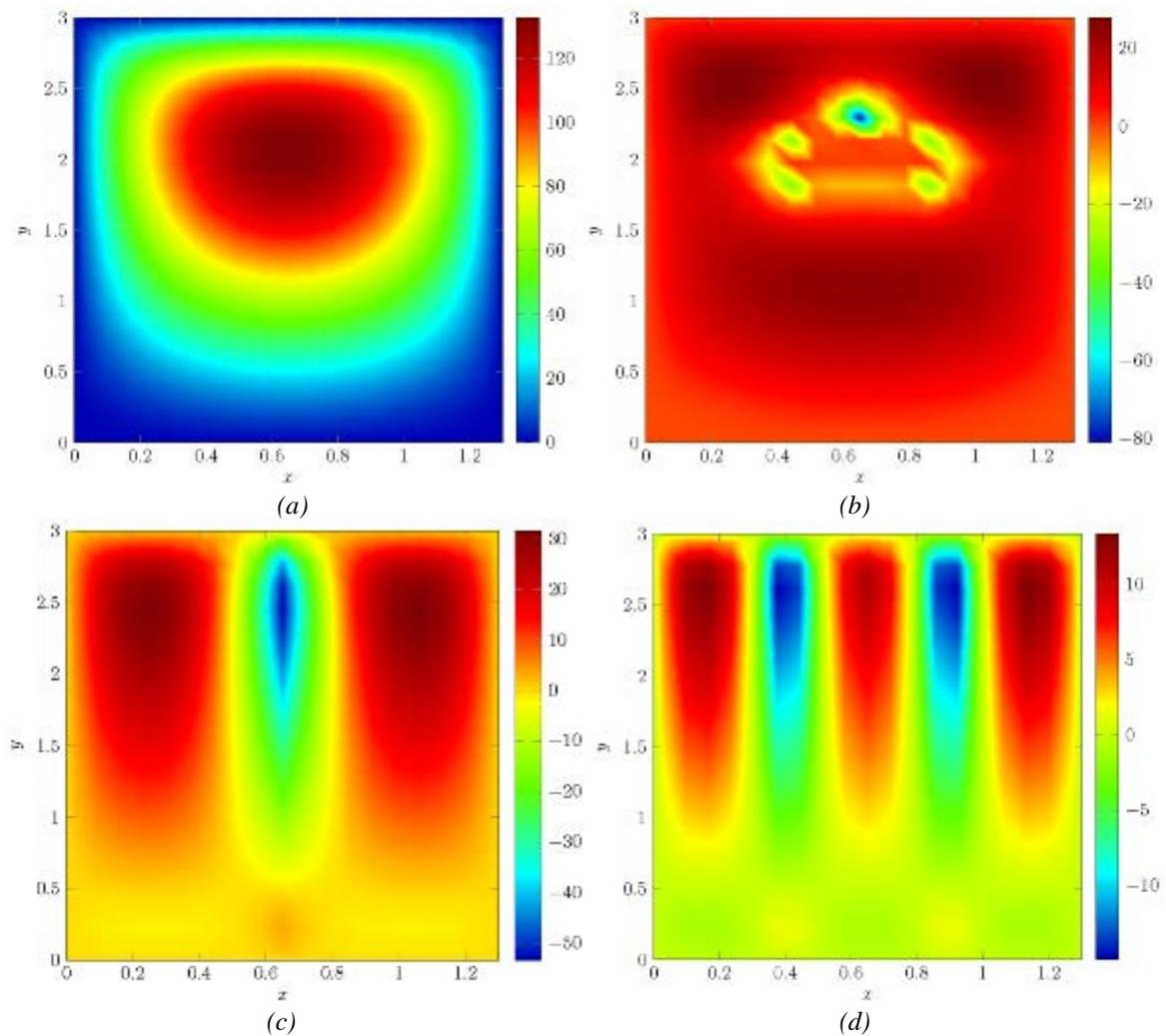
Figure 2. Normal stress distribution  $\sigma_{xx}(x, y)$  of the glasses expressed on MPa for the four cases. (a) Stress with no pillars or stripes, (b) Stress with one pillar, (c) Stress with one stripe, (d) Stress with two stripes.
