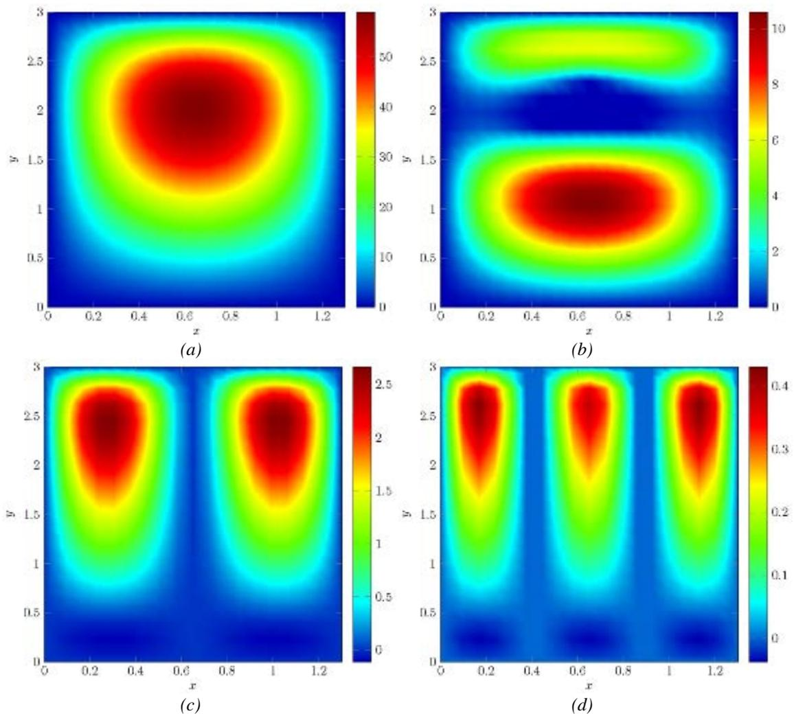
Figure 1. Deflection distribution  $u(x, y)$  of the glass expressed on mm for the four cases. (a) Deflection with no pillars or stripes, (b) Deflection with one pillar, (c) Deflection with one stripe, (d) Deflection with two stripes.
