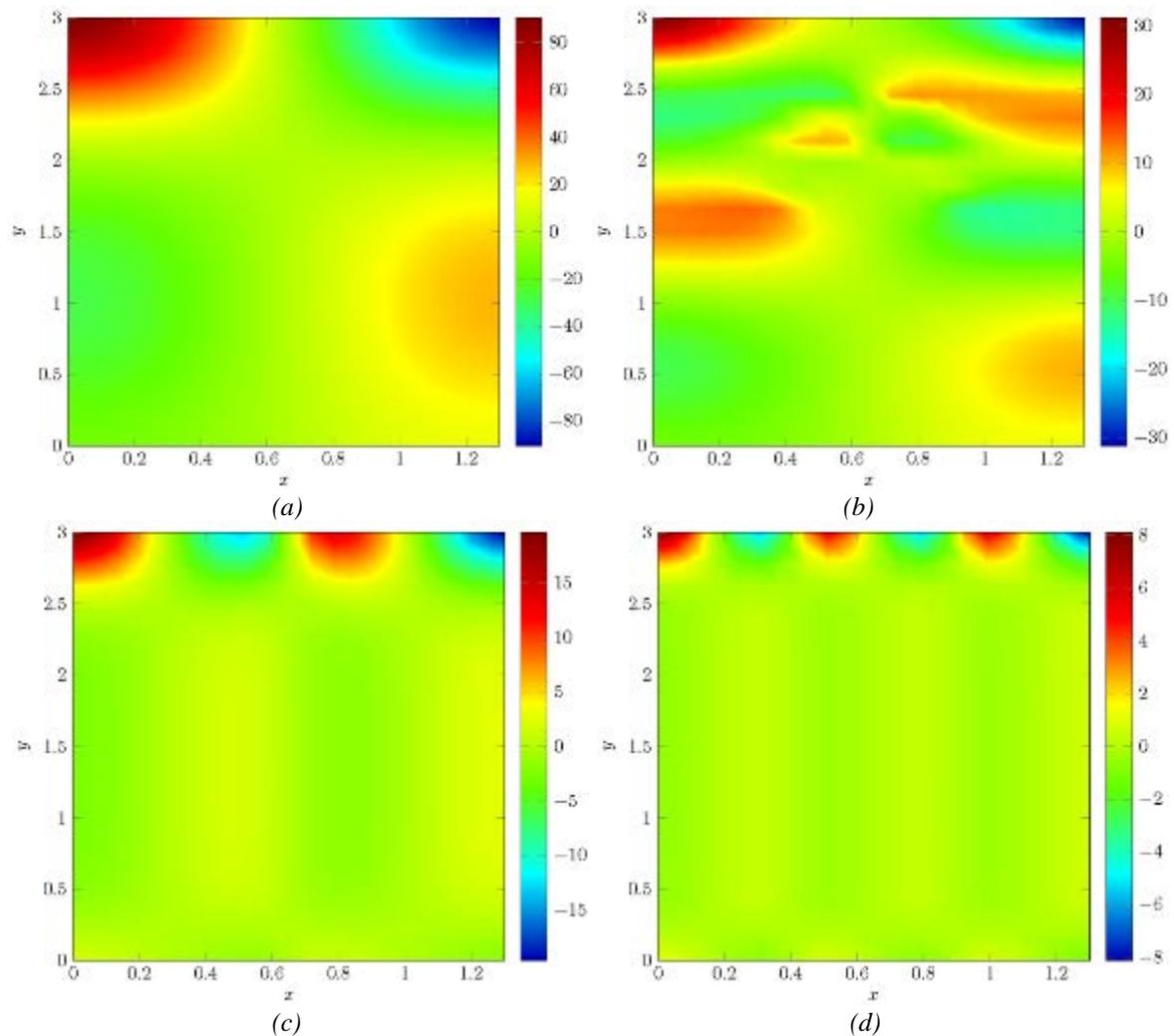
Figure 4. Shear stress distribution  $\sigma_{xy}(x,y)$  of the glasses expressed on MPa for the four cases. (a) Stress with no pillars or stripes, (b) Stress with one pillar, (c) Stress with one stripe, (d) Stress with two stripes.
