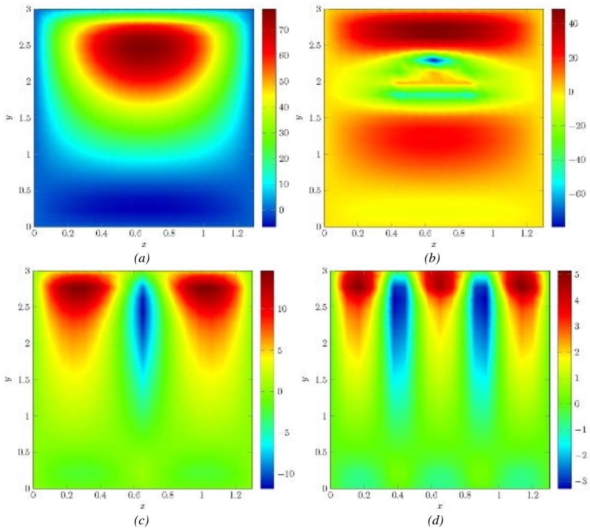
Figure 3. Normal stress distribution  $\sigma_{yy}(x, y)$  of the glasses expressed on MPa for the four cases. (a) Stress with no pillars or stripes, (b) Stress with one pillar, (c) Stress with one stripe, (d) Stress with two stripes.
