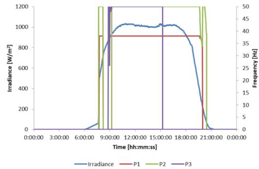
**Figure 7:** Pumps frequency related with the incident irradiance (3rd June 2017)
