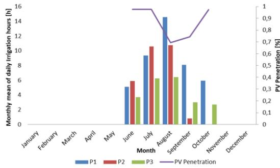
**Figure 6:** Pumps working hours per day in each month and PV penetration
