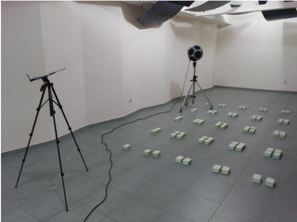
*Image 1: Empty reverberation chamber, with separators of 5 cm.*
