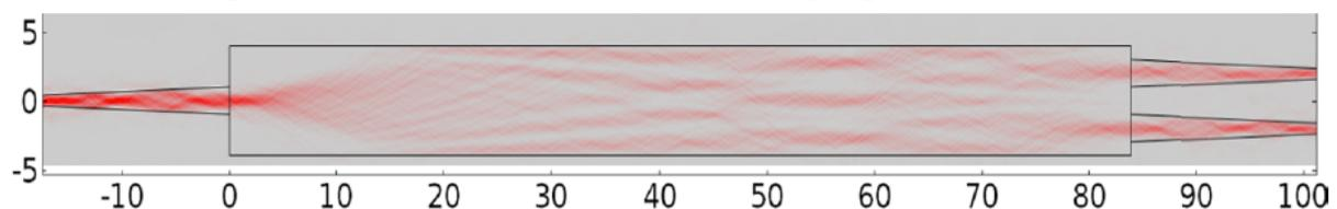
Fig. 1. COMSOL simulation of light intensity distribution in an MMI WG
