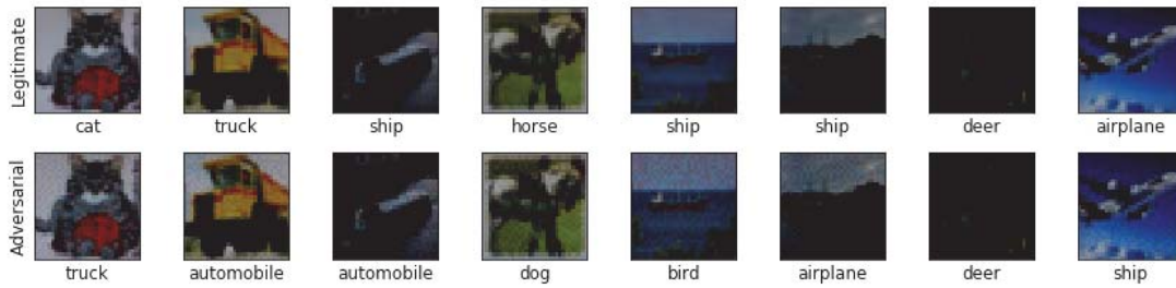
Figure 6.1: Legitimate and adversarial examples from CIFAR-10 dataset used in the experiment. Predicted labels are shown below each image.
