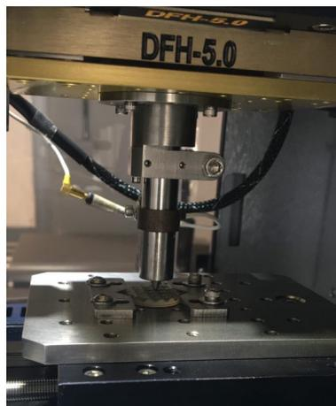
**Figure 1.** Universal mechanical and tribology testing. Sensor DFH- 5.0.
