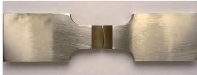
(b) With LSP, PD = 900 cm<sup>-2</sup>, SD = 2.5 mm, crack in the middle of the specimen
