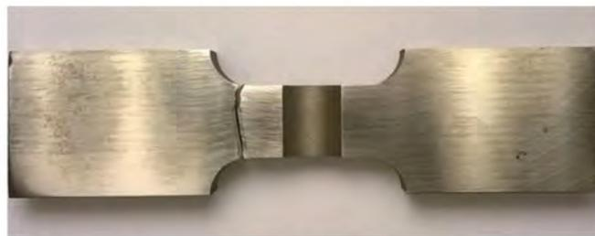
(c) With LSP, PD = 1600 cm<sup>-2</sup>, SD = 2.0 mm, crack at the edge of LSP area
