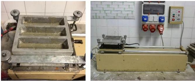
Fig. 7. Filling specimens on mechanical compactor.
