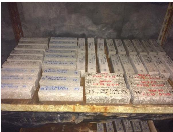
Fig 8. Cured specimens in a humid chamber.
