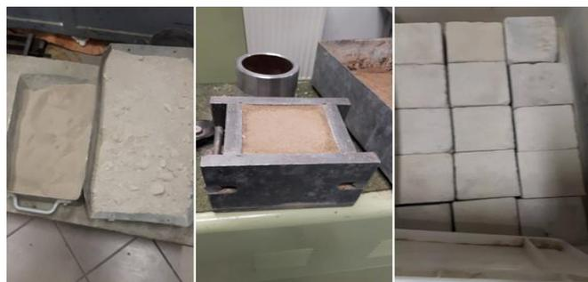
Fig.6. Materials using in experiment and sand- lime samples with recycled fine fraction.
