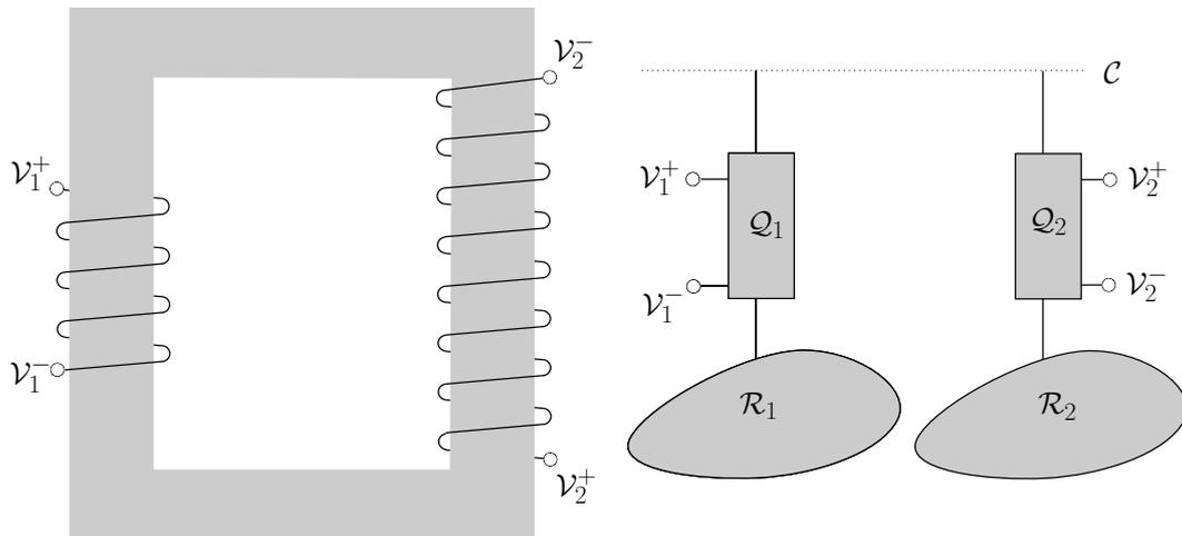
**Figure 8.** The left part of the figure represents a traditional voltage transformer. Magnetic coupling through a ferromagnetic core makes two electrical circuits exchange energy. The relation between the voltages is given by the ratio of the windings. In the right system, the coupling is mediated by a communication line  $C$ . Two nodes, each one with a Quiieg share the qubits that travel through  $C$ . By setting the  $p_a$  parameter, the voltage difference at each node is selected.
