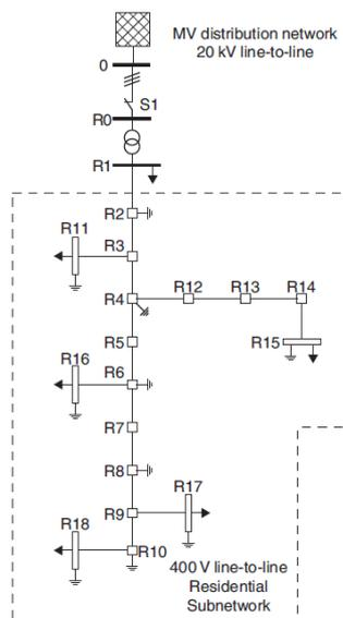
Fig. 1. CIGRE European Low Voltage Distribution Test Network
