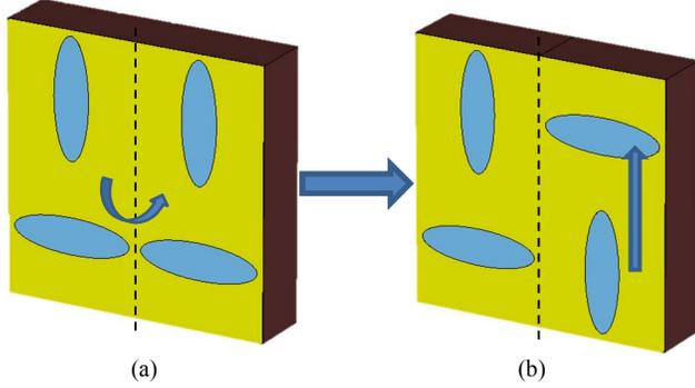
Fig. 4. The non-glide-symmetric structure in Fig. 2 (c) mirrored using a different symmetry axis (a). The new glide-symmetric structure (b) is obtained from (a) after applying a translation.
