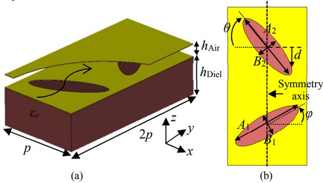
Fig. 1. Unit cell of the proposed structure and parametrization. View in perspective (a) and top view without the top metal plate (b).
