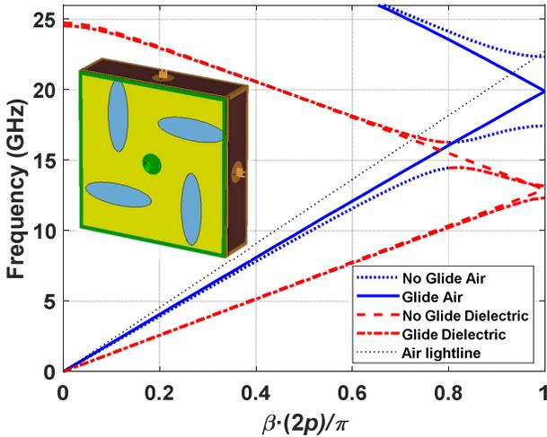
Fig. 5. Dispersion diagram of the structure in Fig. 4(b) with regenerated symmetry compared to the original non-glide-symmetric structure in Fig. 2(c).
