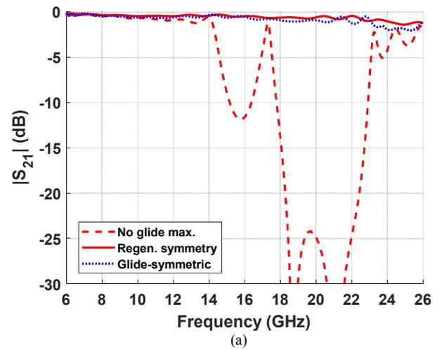
Fig. 7. Simulated S parameters of the designs in Fig. 6 (a-c). The  $S_{21}$  parameters are shown together with the dispersion diagrams to compare the position of the stop-bands (a). The  $S_{11}$  parameters are shown in (b).
