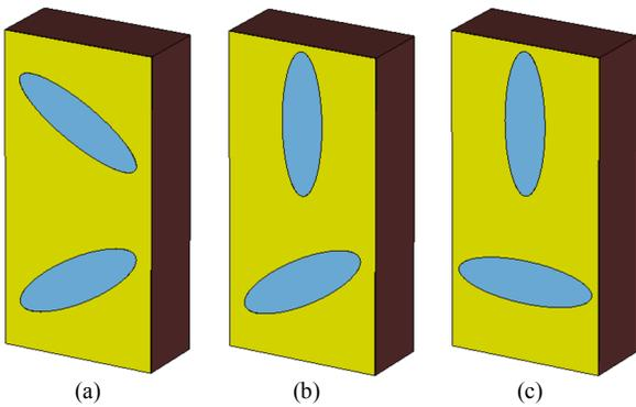
Fig. 2. Unit cell of a glide-symmetric (a), non-glide-symmetric (b) and maximally non-glide-symmetric (c) structures.
