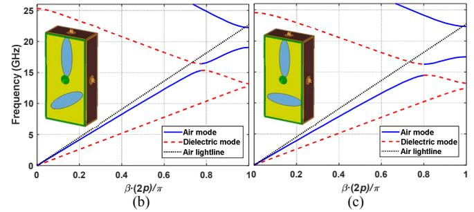
Fig. 3. Dispersion diagrams for three configurations of the unit cell: glide-symmetric (a), non-glide-symmetric (b) and maximally non-glide-symmetric (c).
