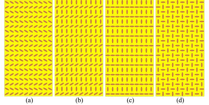
Fig. 6. Full designs with 10x10 unit cells of a glide-symmetric (a), non-glide-symmetric (b) and maximally non-glide-symmetric (c) structures and 5x10 unit cells of the regenerated glide-symmetric design (d).
