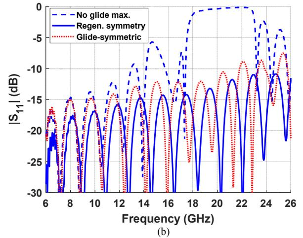
Fig. 8. Simulated S parameters of the design with regenerated symmetry in Fig. 6 (d) compared to the results of the original glide and non-glide designs. The  $S_{21}$  parameters are shown in (a) and the  $S_{11}$  parameters are shown in (b).
