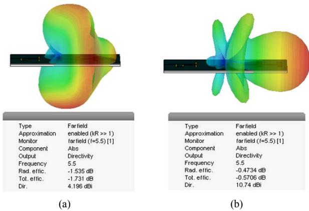
Fig. 4. 3D farfield pattern as a function of the graphene sheet resistance:  $R_s = 6 \Omega/\text{sq}$  (a) and  $R_s = 2580 \Omega/\text{sq}$  (b).
