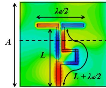
Fig. 2. Electric field distribution over the printed dipole and the balun. The dashed line delimits the ground plane size.
