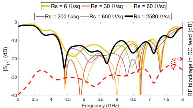
Fig. 6. Reflection coefficient as a function of the graphene sheet resistance and the RF blockage level in the DC bias point.
