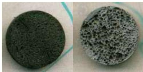
**Figure 1.** Aluminum foams of approximately 1 and 2 mm average pore size manufactured by the powder metallurgical technique
