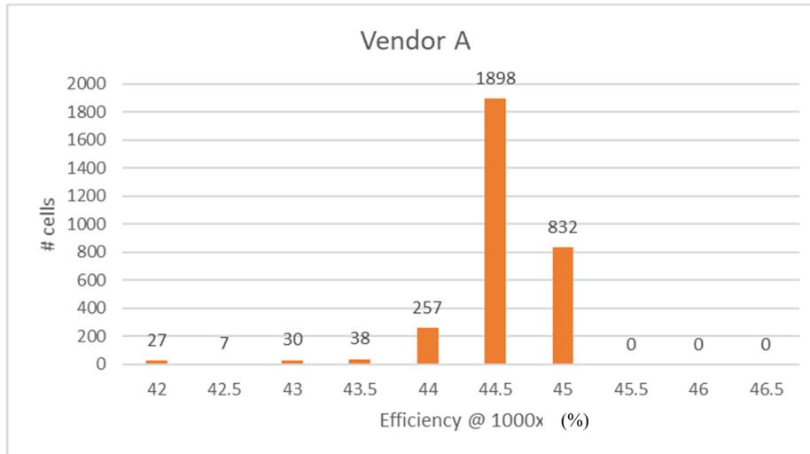
**FIGURE 1.** Cell efficiency distribution histogram for one of the types of solar cell chosen for this project. The choice of cell has clearly enabled a much higher efficiency to be achieved compared with those used in Gen 1 of the module design (typically ~37%).
