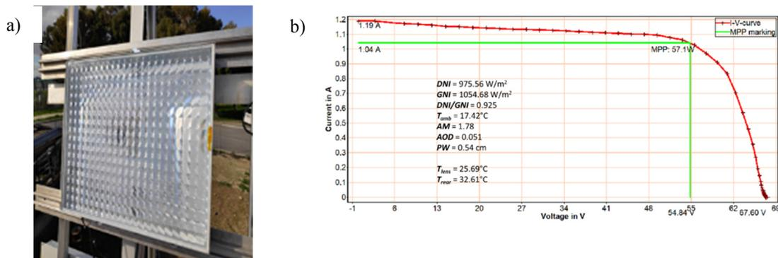
**FIGURE 4.** a) Image of Gen 1 module on tracker at UCY in Cyprus, and b) Initial on-sun module IV curve of this module, confirming previous performance
