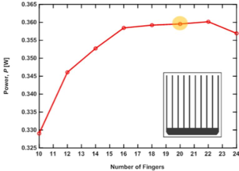
**FIGURE 2.** Results of the optimization process for the front grid considering the irradiance distribution of our optical train and a solar cell structure from Solar Junction Corporation (USA).
