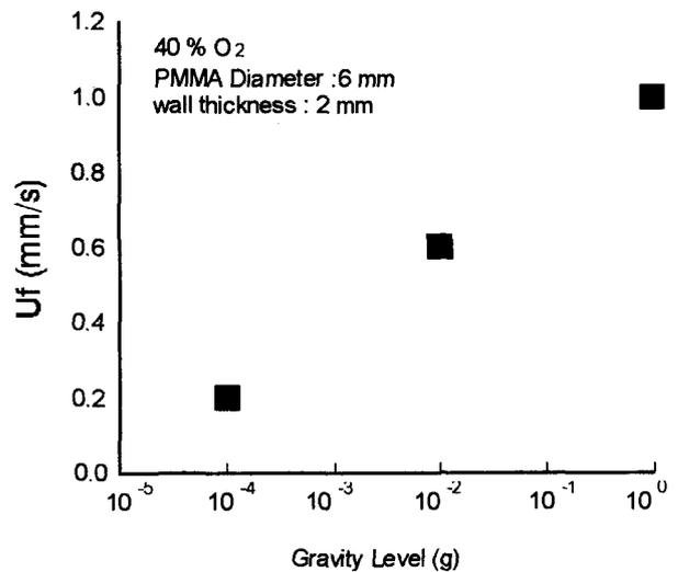
Fig. 6.- Influence of gravity level on flame spread velocities. Y<sub>O<sub>2</sub></sub>= 40%, diameter=6 mm, thicknes=2 mm
