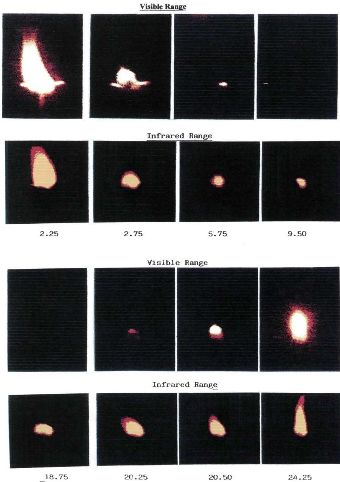
Fig. 2.- Simultaneous video colour and infrared photographs of a PMMA Cylinder burning at reduced gravity. [(Times from ignition (sec)) ( $Y_{O_2} = 23\%$ ); (small differences in time of the order of 0.2 s between IR and visible photographs might exist).
