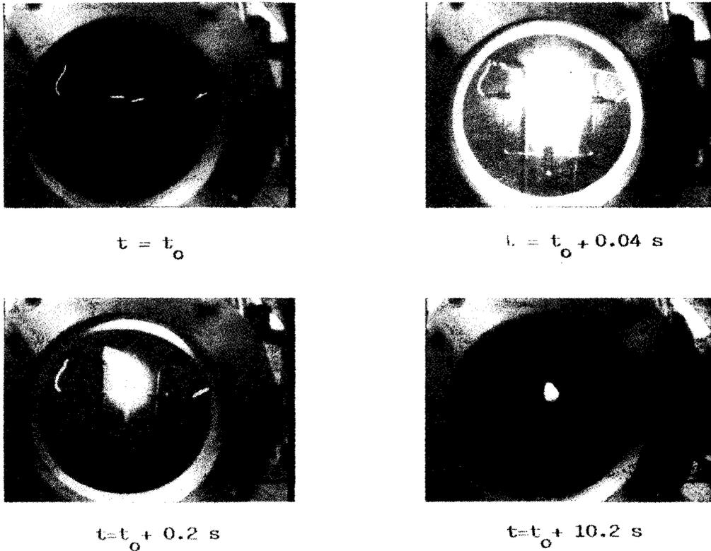
Fig. 4 Ignition and combustion processes.  $Y_{O_2} = 40\%$ , thickness = 2 mm
