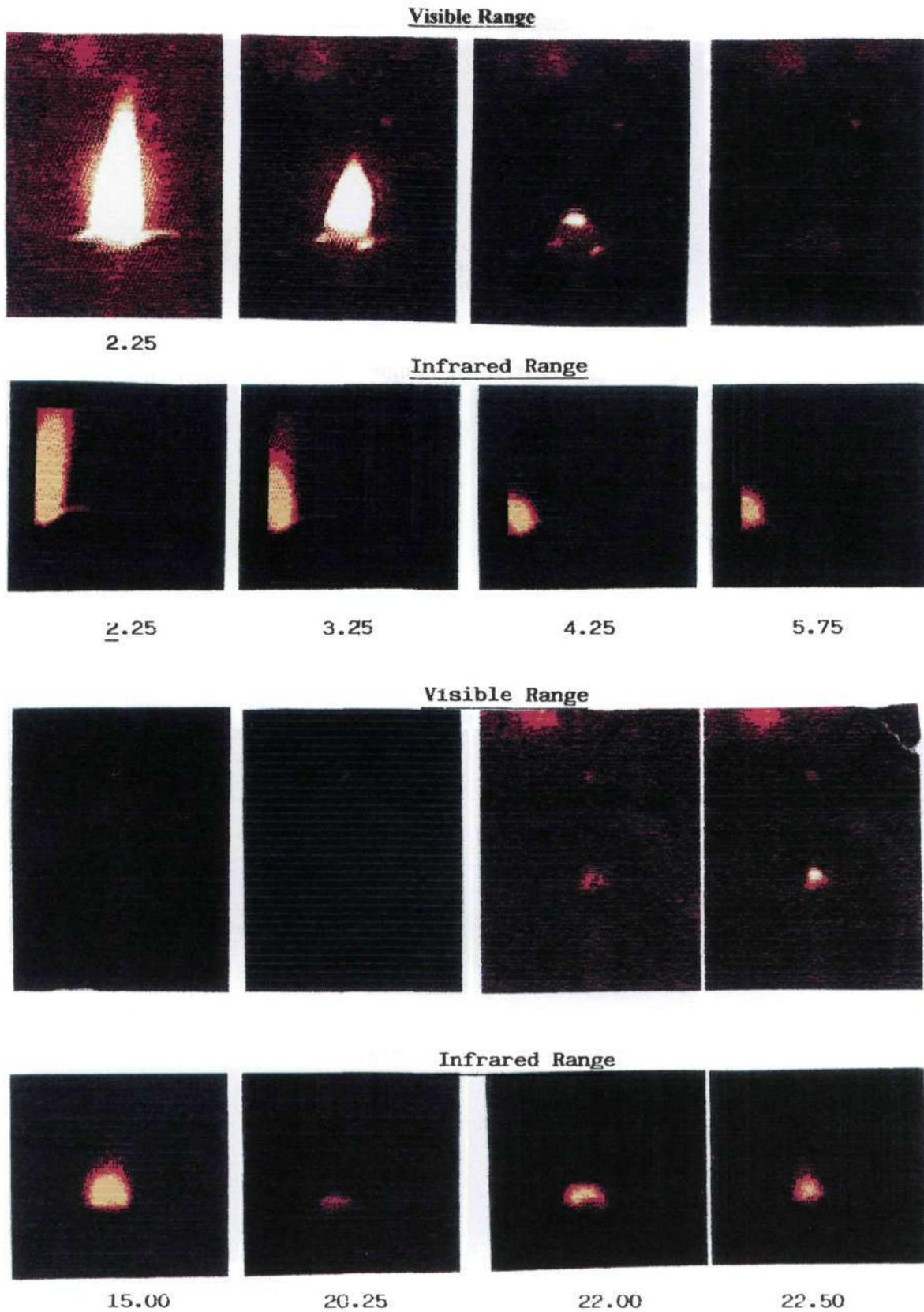
Fig. 3.- Simultaneous video colour and infrared photographs of a PMMA Cylinder burning at reduced gravity. [(Times from ignition (sec))(Y<sub>O<sub>2</sub></sub> = 21%); (small differences in time of the order of 0.2 s between IR and visible photographs might exist).
