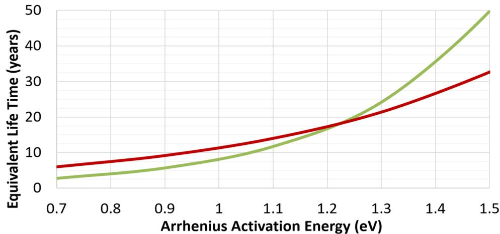
**FIGURE 2.** Estimated equivalent lifetime for CoCs, if the product pass this test, vs. activation energy for the test “High temperature with current injection test” (green line 400 hours at 130 °C and alternatively red line 2500 h at 110 °C with 0.5 Isc current injection) considering a CoC operation temperature of 85 °C.
