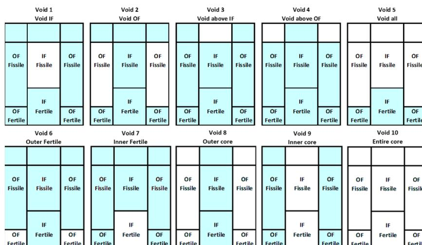
**Figure 1: Sodium void zones and corresponding case numbers**
