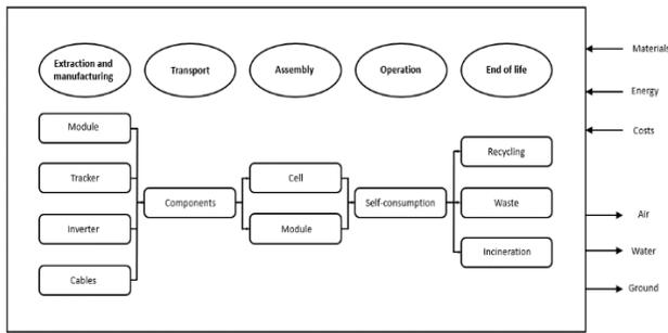
**Figure 1.** Life cycle processes, system boundaries and flows considered in the LCI of the micro-CPV module
