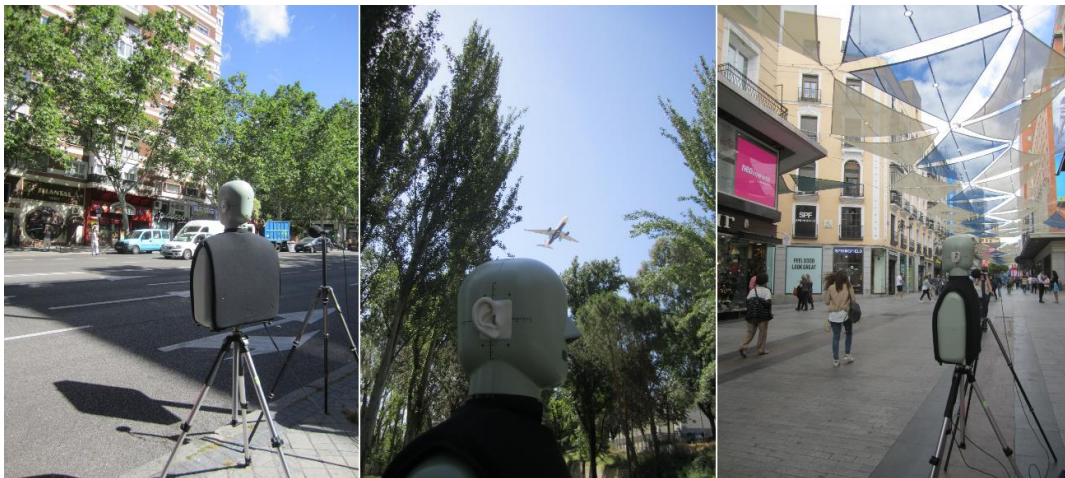
Figure 1: Dummy Head during the recording of the urban sources of noise. Left, urban traffic. Middle, flyover of aircrafts. Right, pedestrian noise.
