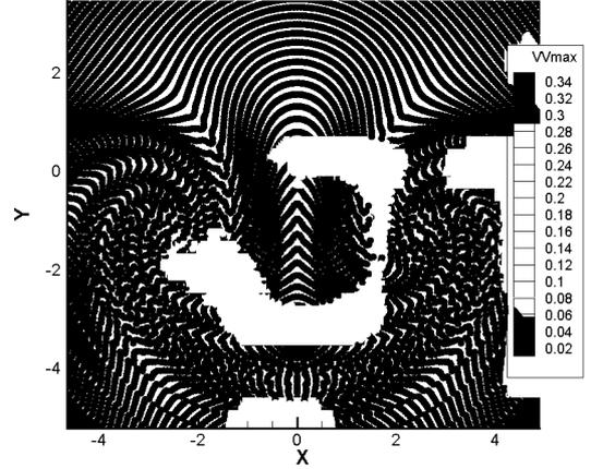
Fig. 7. Snapshot of the velocity magnitude at time  $t = 14s$  calculated by ISPH(TVT). $nr = 186$  and  $h = 1.8dx$
