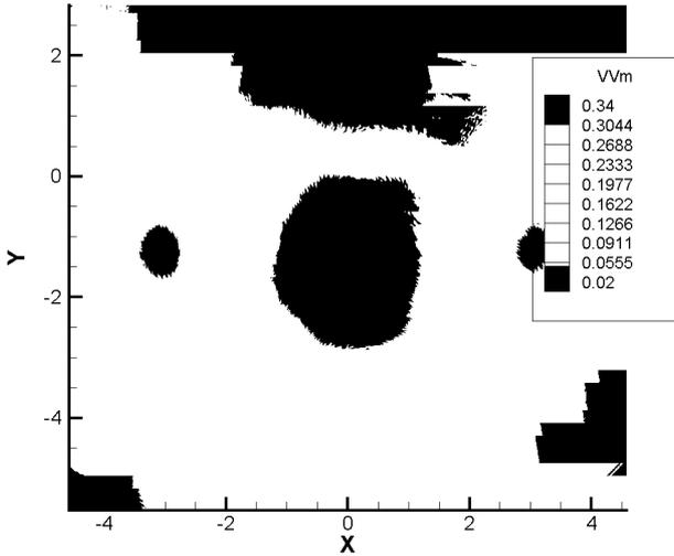
Fig. 3. Snapshot of the velocity magnitude at time  $t = 14s$  calculated by WCSPH(TVT),  $nr = 526$  and  $h = 1.33dx$
