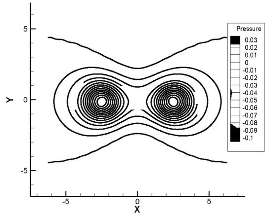
Fig. 10. Pressure field at  $t = 1$  for  $Re = 100$  calculated by the ISPH code.
