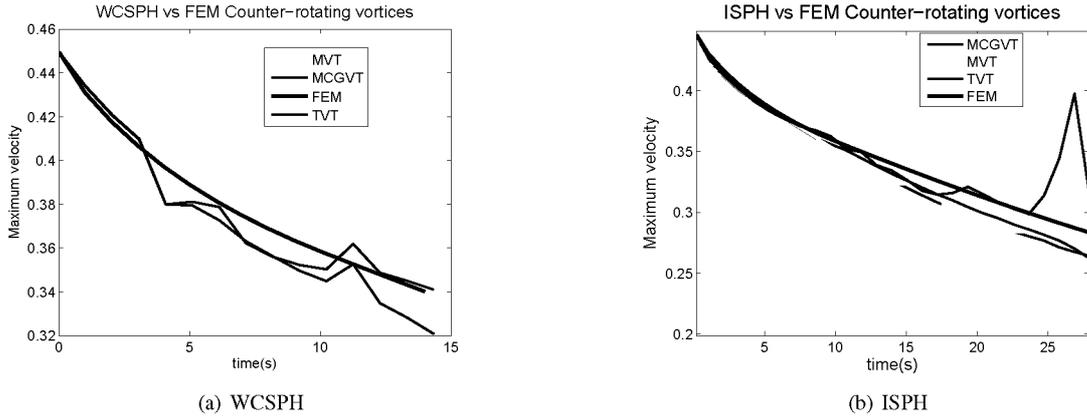
Fig. 8. Comparison of the evolution of the maximum of the velocity performed by the WCSPH(nr=526) and the ISPH(nr=126) and different viscosity models.
