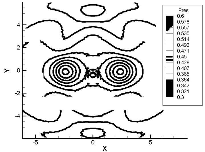
Fig. 5. Pressure field at  $t = 1$  for  $Re = 100$  calculated by the WCSPH code.
