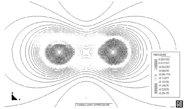
Fig. 4. Pressure field at  $t = 1$  for  $Re = 100$  calculated by the ADFC-FEM code
