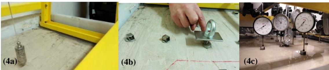
Figure 4. (4a) Detail of the plumb line and levelling layer; (4b) placement of the anchor and profiles; and (4c) detail of dial gauges and water level.
