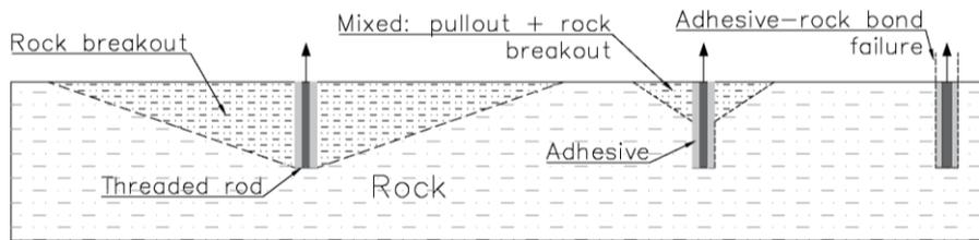
Figure 1. Principal modes of failure of adhesive anchors.
