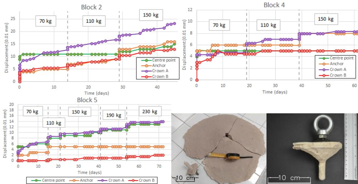
Figure 5. Results of the three creep tests and examples of types of obtained failures.
