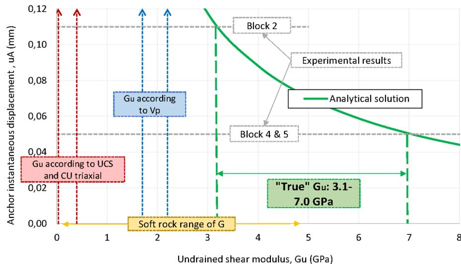
Figure 6. Variation of the instantaneous displacement as a function of the shear modulus.
