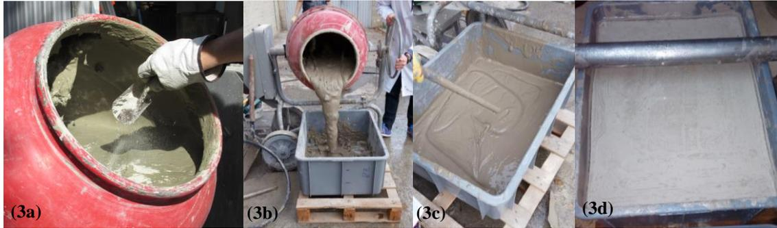
Figure 3. (3a) Optimal mixing process; (3b) pouring of the first layer; (3c) appearance after the vibration of the first layer; and (3d) final appearance after 72 h of setting in a humid chamber.
