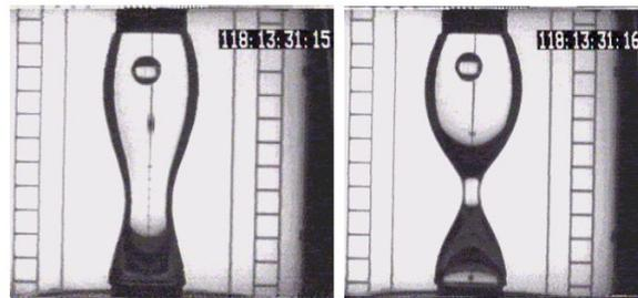
**Figure 1** 1993 Spacelab-D2 mission (experiment STACO), breaking of a cylindrical volume liquid<sup>24,25</sup>.
