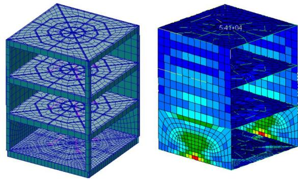
**Figure 4: FEM model of the UPMSat-2 by MUSE students (left), and its Nastran-Patran<sup>®</sup> calculation (right).**
