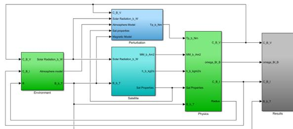
**Figure 8: ADCS model of UPMSat-2 in Matlab/Simulink.**
