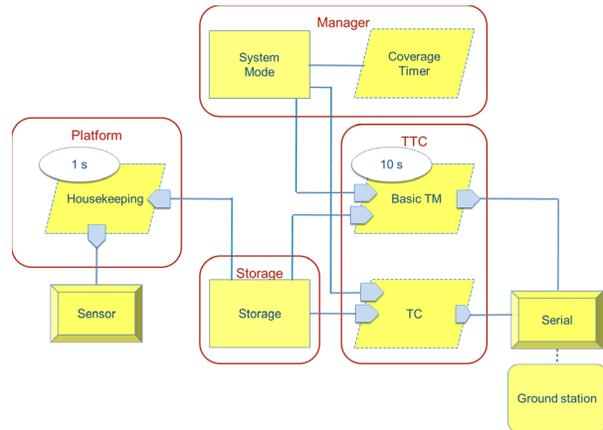
**Figure 7: Simplified scheme of the UPMSat-2 on-board software.**
