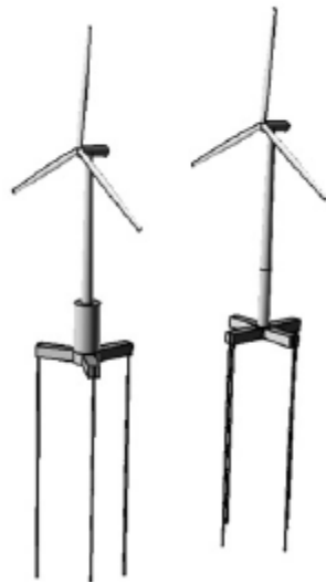
Fig. 1.12 Schemes of TLPWT showing the variation on design variables: sea-surface mast diameter, pontoon size and number of tension legs, Bachynski and Moan, (2012).
