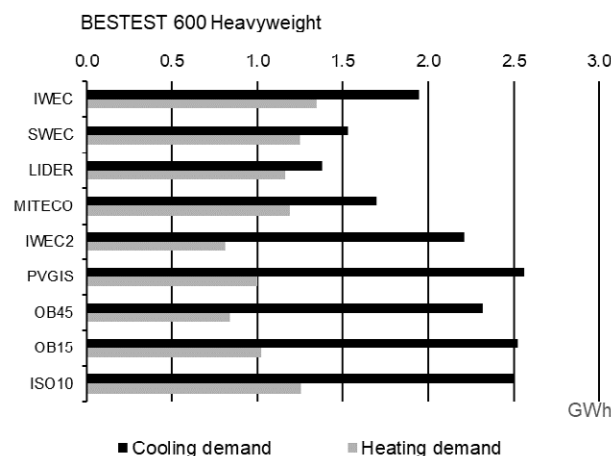
Figure 1: Cooling and heating energy demand produced with each weather file of Madrid for the BESTEST 600.
