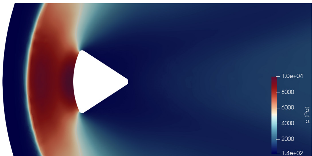
Figure 5.52. Shock capturing: Detailed view of the pressure distribution near the shock wave with p = 2 , for the real inflow conditions before the shock wave and AoA = 0^\circ .
