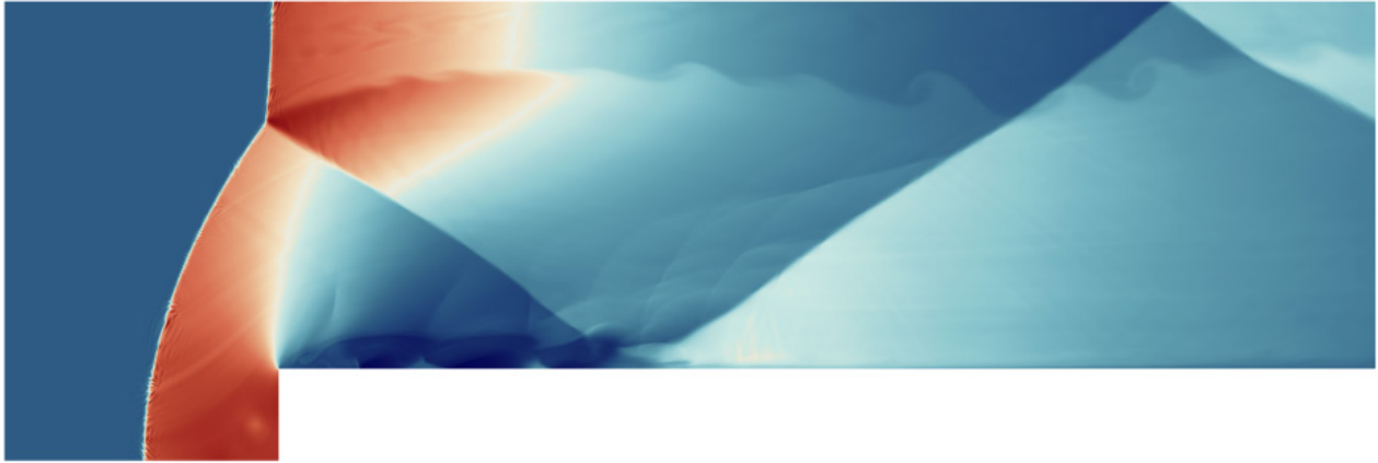
Figure 3.10. Facing forward step case at \tau = 10 with an incoming flow at Mach 3 and 3653 elements with polynomial degree N = 7 . [11]
