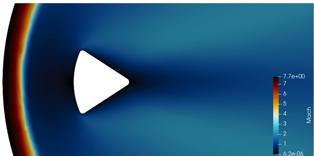
Figure 5.48. Shock capturing: Detailed view of the Mach number distribution near the shock wave with p = 2 , for the real inflow conditions before the shock wave and AoA = 0^\circ .
