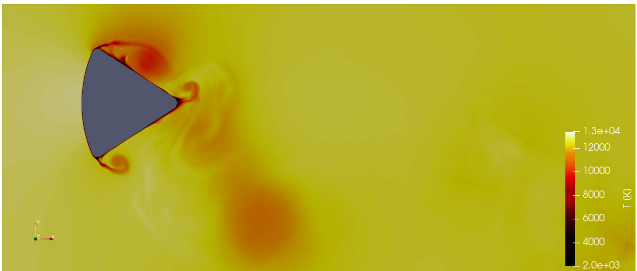
Figure 5.10. Isothermal capsule: Snapshot of the temperature distribution in the fluid domain with p = 2 , for the inflow conditions after the shock wave and AoA = -18^\circ .
