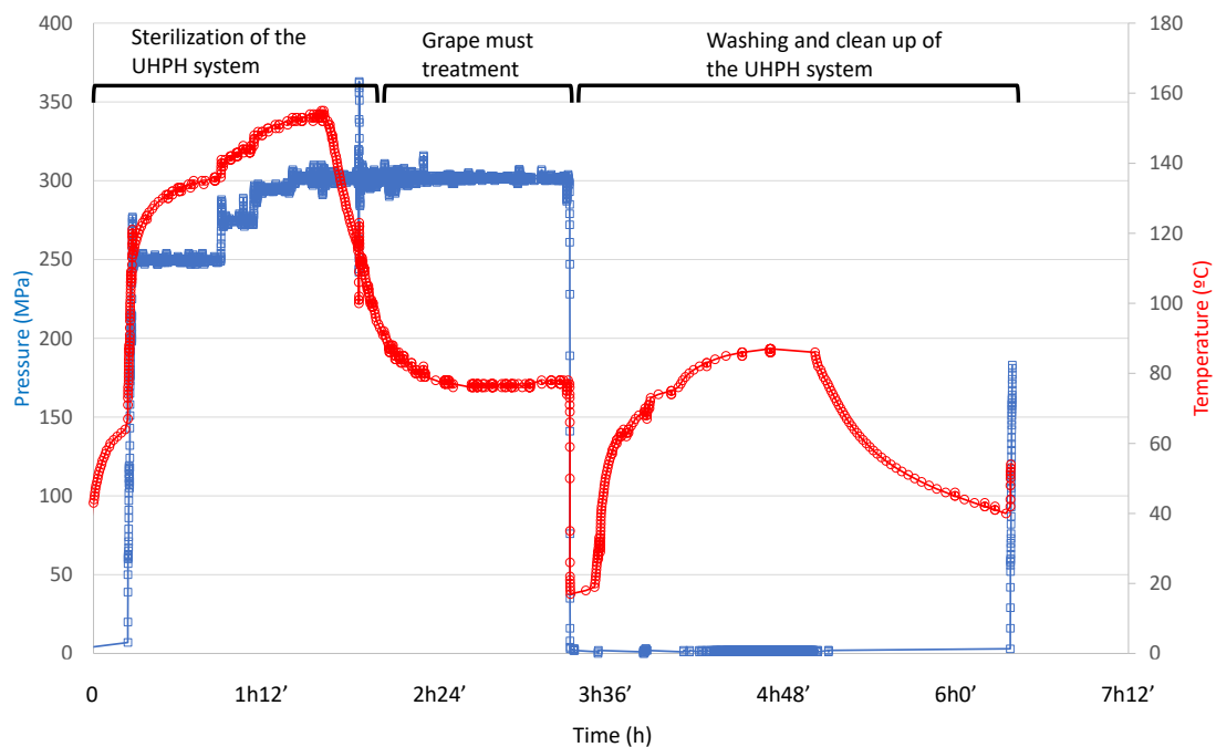
Figure 1. Pressure (MPa): blue dots; in-valve temperature (°C): red dots.
