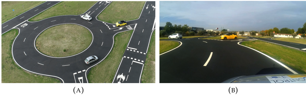
FIGURE 8.38: Demonstrator status during the merging maneuver. (A) Aerial view. (B) Lag vehicle's point of view.
