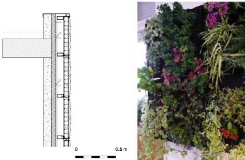
Fig.4: Prototype Built and Constructive Section of the Solution
