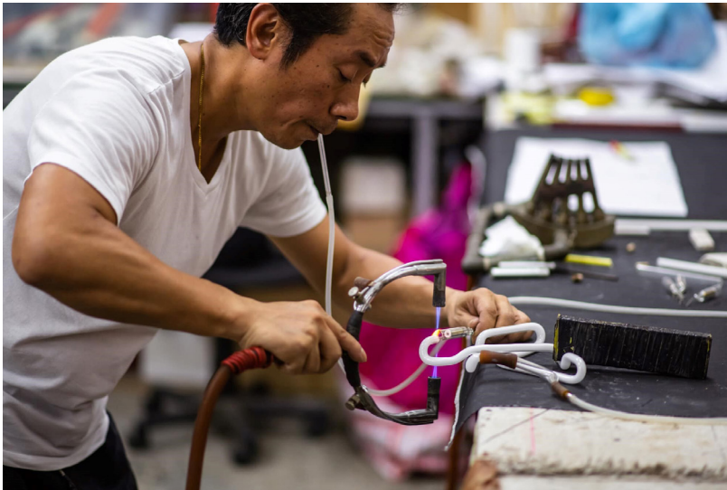
Fig. 296. An operator manually crafts a commercial neon sign, 2019, Hong Kong. Source: Street Sign Hong Kong.
