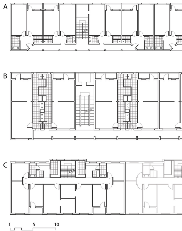
Fig. 268. Interior layouts of three Hanoi communal apartment buildings: Kim Liên (a), Trung Tu (b) and Nguyễn Công Trù (c). Source: author, based on plans and drawings gathered by Geertman, Stephanie, 'The Self-Organizing City in Vietnam; Processes of Change and Transformation in Housing in Hanoi' (Technische Universiteit Eindhoven, 2007).
