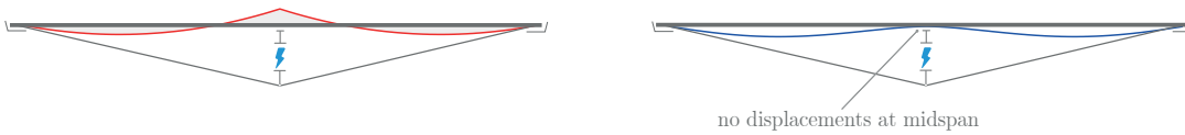
Figure 4.1: Bending moments (left, in red) and displacements (right, in blue), in the deck for the different load conditions.
