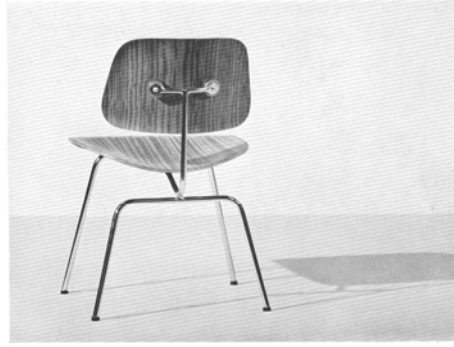
Body-curved plywood seat and back are attached to a handsome tubular steel frame by means of rubber cushions in order to impart sufficient pliability.
