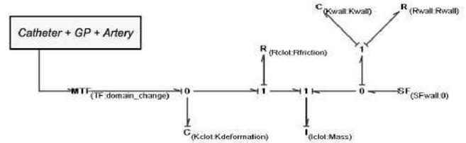
Figure 4. Modelling clot components by Bond Graph technique.
