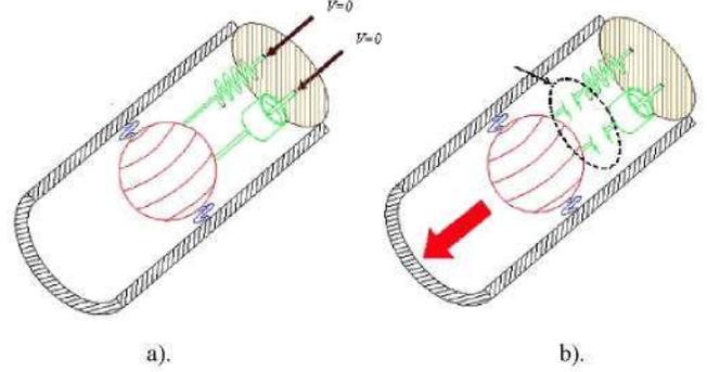
Figure 3. Spring-damper system. a).  $F < \text{Adhe. force}$ . b).  $F \geq \text{Adhe. force}$ .
