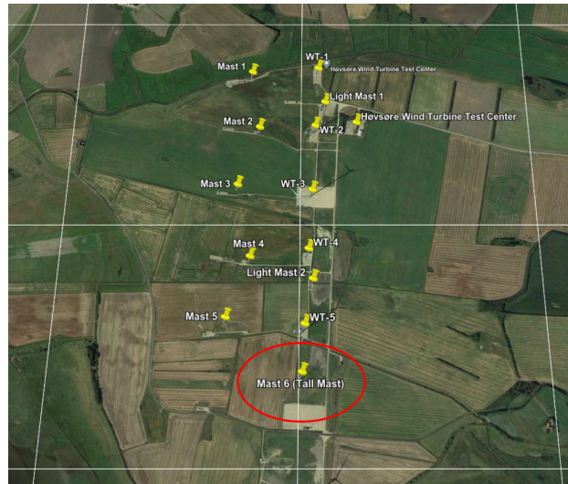
Figure 8.34: A screenshot from Google Earth satellite imagery of Høvsøre, Denmark, with wind turbines and experimental means indicated by yellow pins. The Høvsøre mast is encircled by a red ellipse. The white solid boxes indicate the boundaries of the finest WRF grid projected onto the test site ( \Delta x = \Delta y = 1 km).
