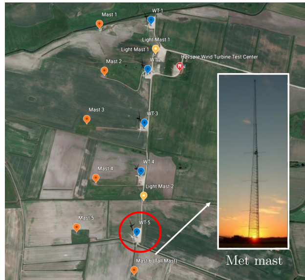
Figure 8.31: A screenshot from Google Earth satellite imagery of Høvsøre, Denmark. The layout of the Høvsøre site shows the locations of the wind turbines and the instrumentation installed in the test site. The wind turbine considered in this work is encircled by the red circle. Experimental data was collected from a 116.5 m met mast shown in a white box. Met mast locations are marked by orange and yellow pins, whereas wind turbine locations are indicated by blue pins.
