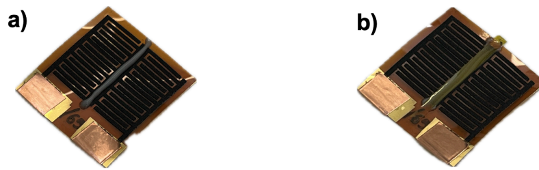
Figure 39: Examples of 2 V supercapacitor modules. (a) 2 V microsupercapacitors separated with an epoxy string. (b) 2 V microsupercapacitors separated with a polyimide film.
