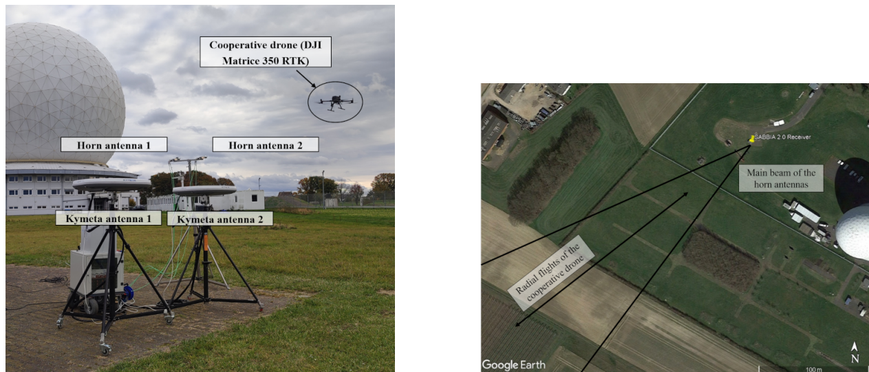
Figure 6.32: Measurement scenario to validate the target detection capabilities: Picture of the setup including the cooperative drone, two Kymeta antennas used as reference channels and two surveillance horn antennas used as surveillance channels (left), and satellite view of the area indicating the pointing and monitored sector of the horn antennas in which radial flights were performed by the cooperative drone.
