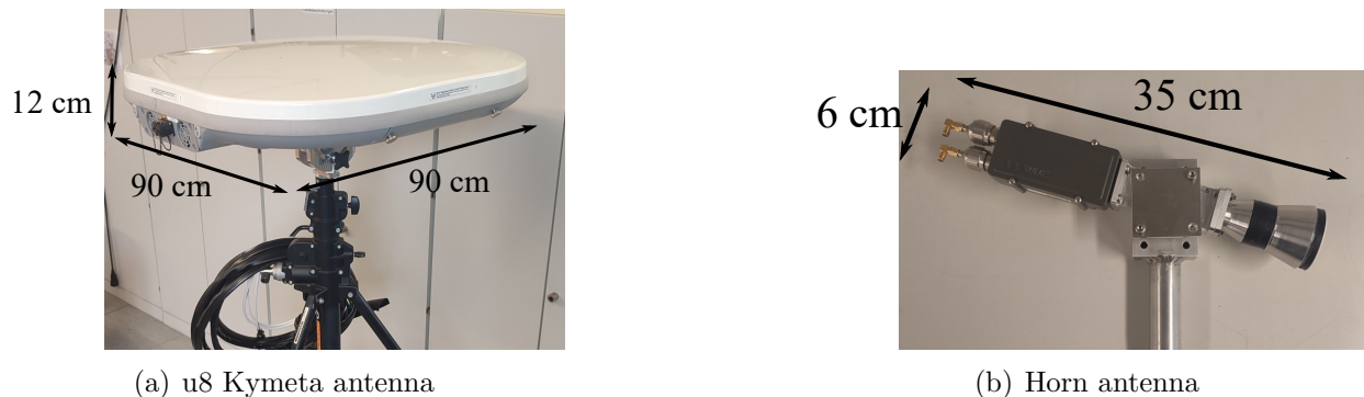
Figure 6.3: Antenna setups used for the measurement campaign and associated dimensions.
