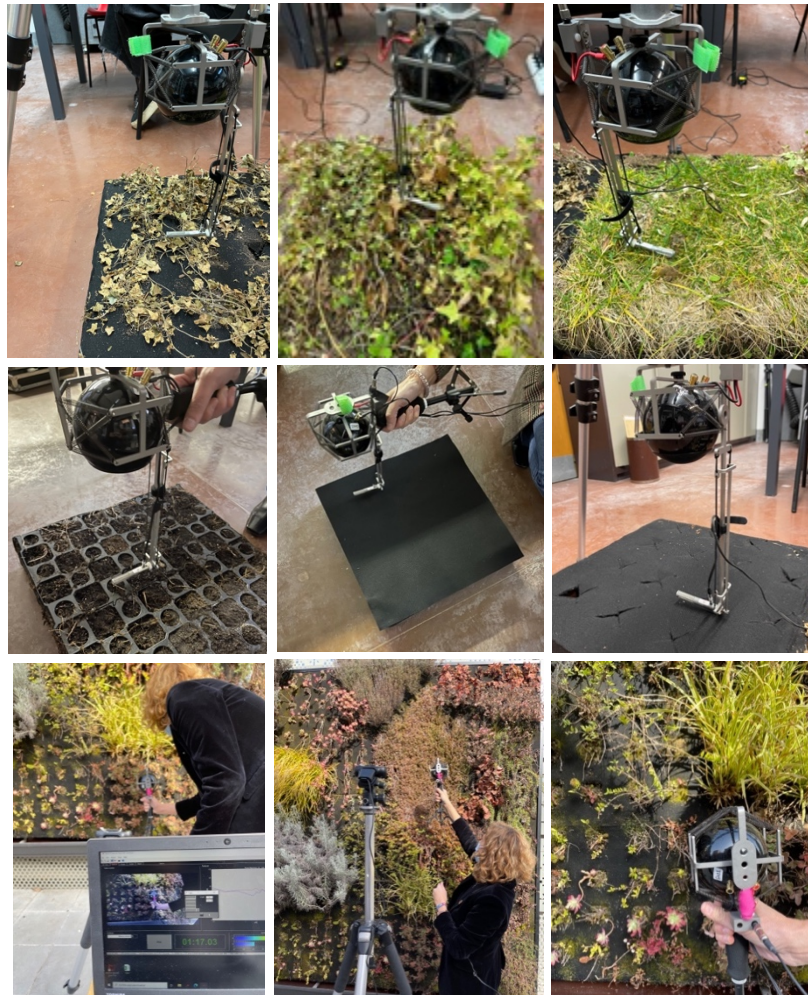
Figure 41: Sound absorption measurements in laboratory and in-situ green wall.
