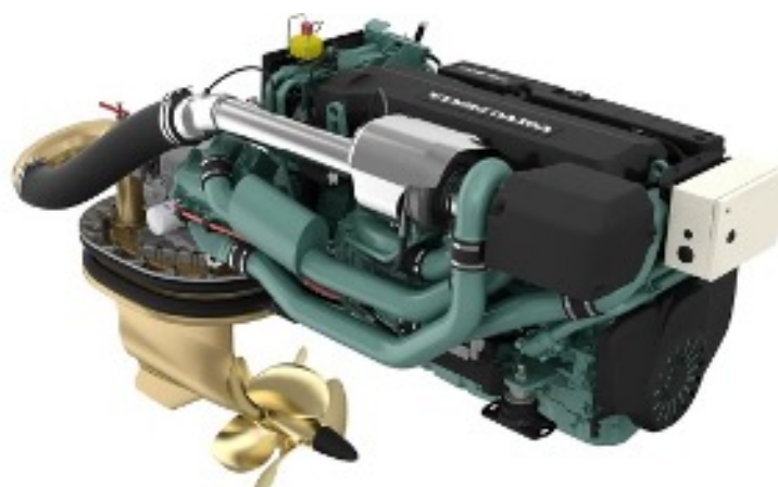
Figura 6.5: Motor Volvo Penta IPS
