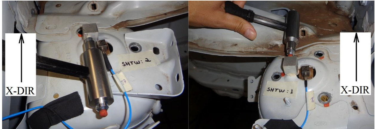
Figure 25. Impact hammer x-dir load on front left and front right body structure shock tower.
