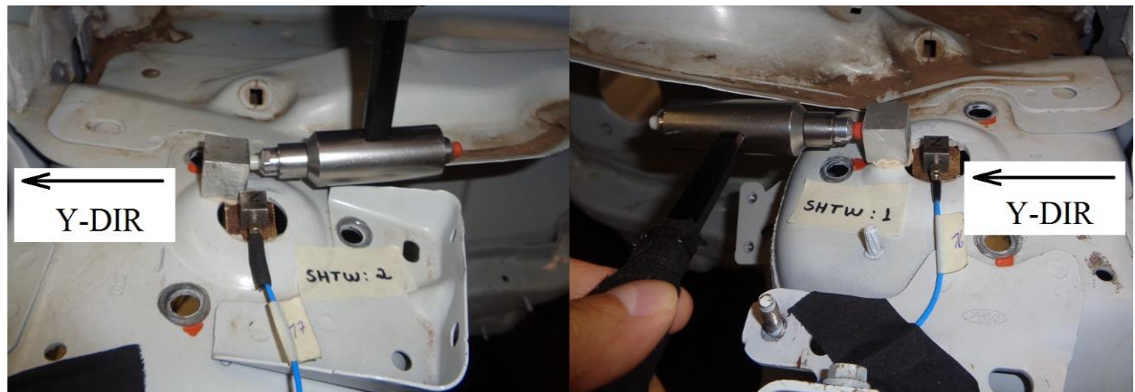
Figure 26. Impact hammer y-dir load on front left and front right body structure shock tower.
