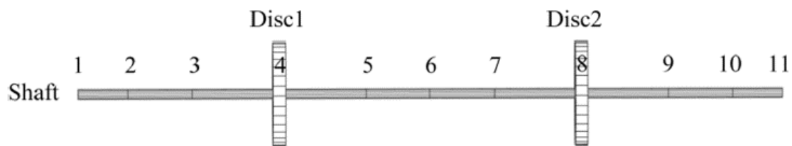
Figure 15. Dual rotor-discs FE model [19]
