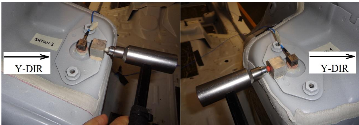
Figure 29. Impact hammer y-dir load on rear left and rear right body structure shock tower.
