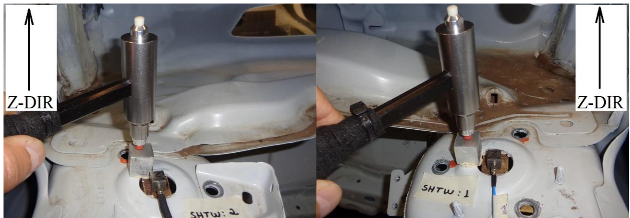
Figure 27. Impact hammer z-dir load on front left and front right body structure shock tower.
