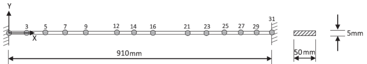
Figure 10. Fixed-fixed beam structure [16]
