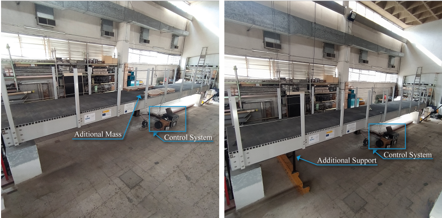
(a) Additional mass. (b) additional support.
