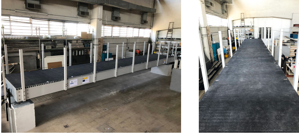
Figure 3.7: FRP footbridge at the Laboratory of Structures of the Technical University of Madrid.
