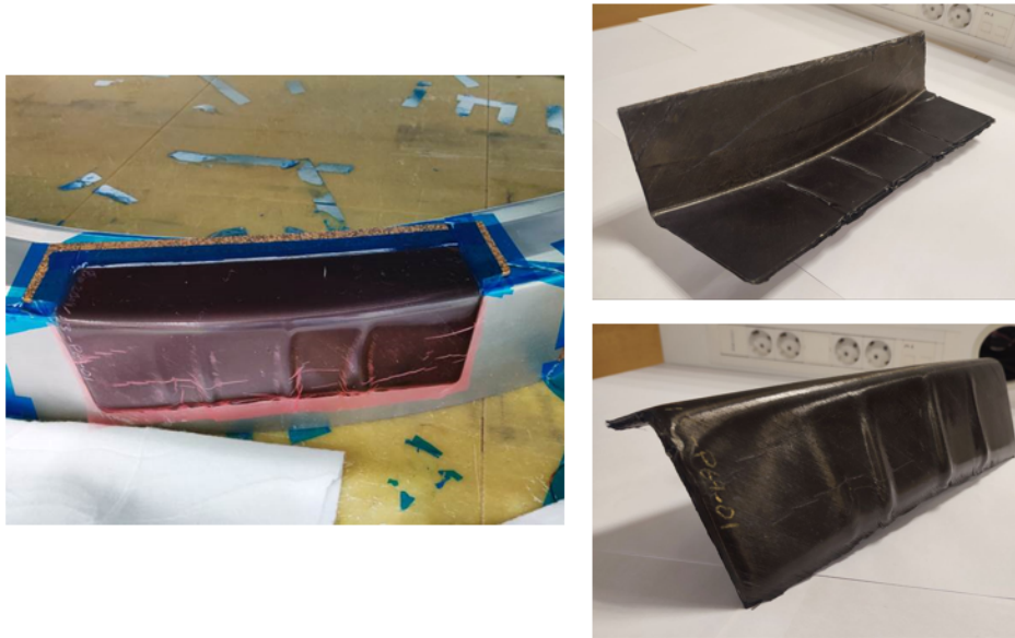
Figure 4.13: Experimental thermoforming production process of prepreg with wrinkle formation
