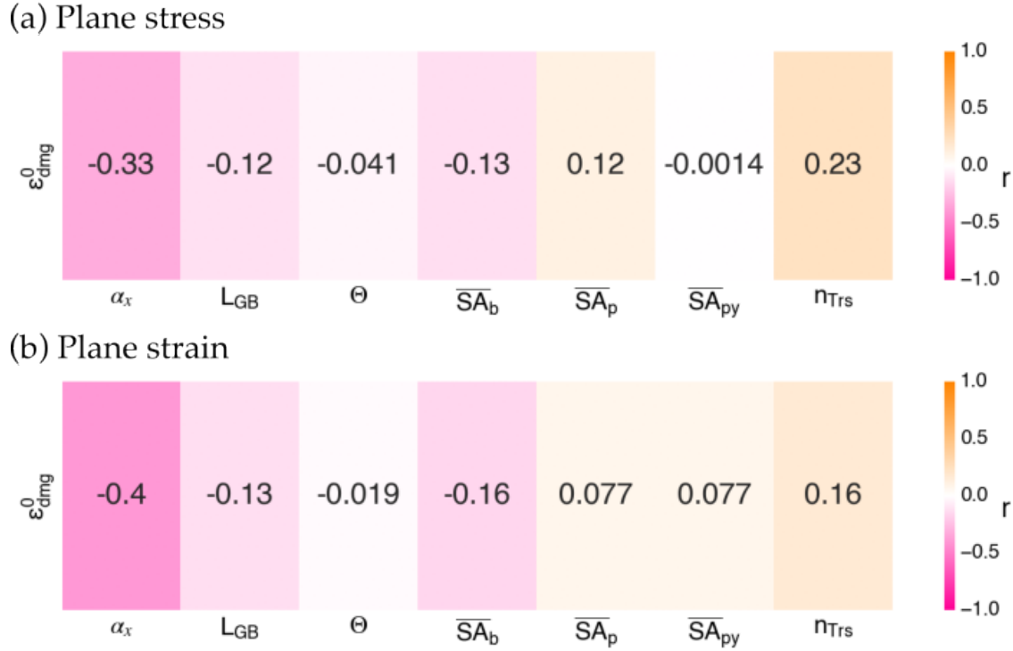
Figure 7.23: Pearson correlation matrix for GB fracture in the Mg foils with strong basal texture. (a) Plane stress, (b) plane strain.
