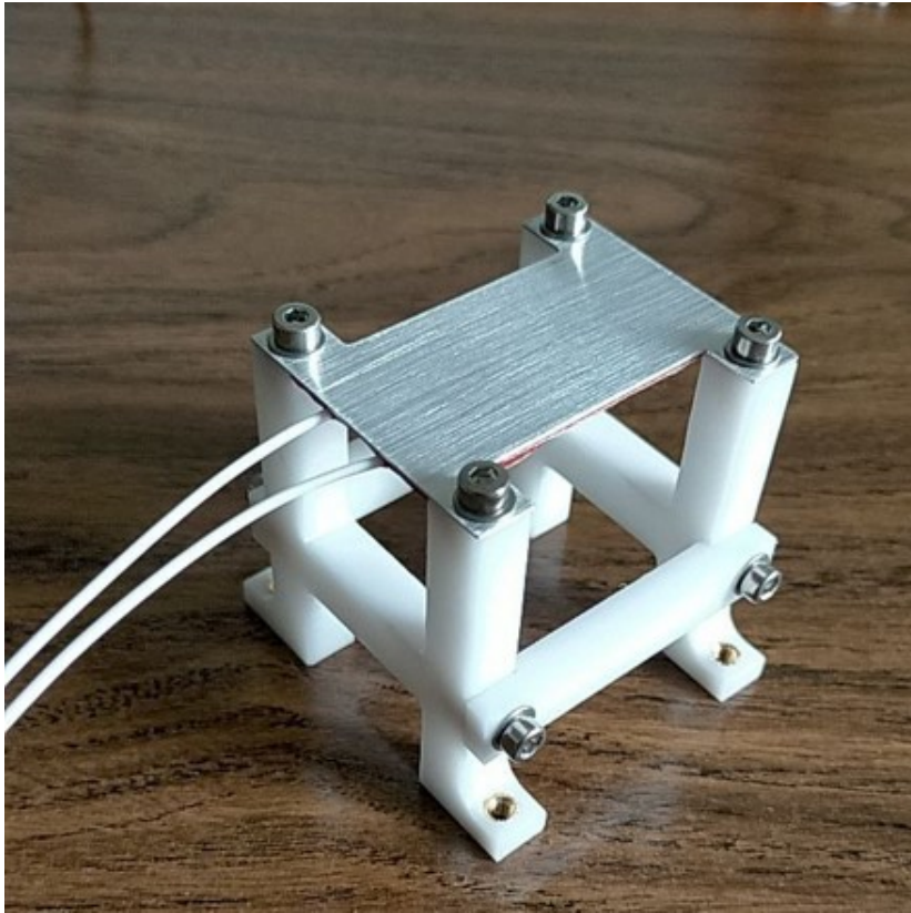
Figure 4.2: Delrin support of the heated plate.
