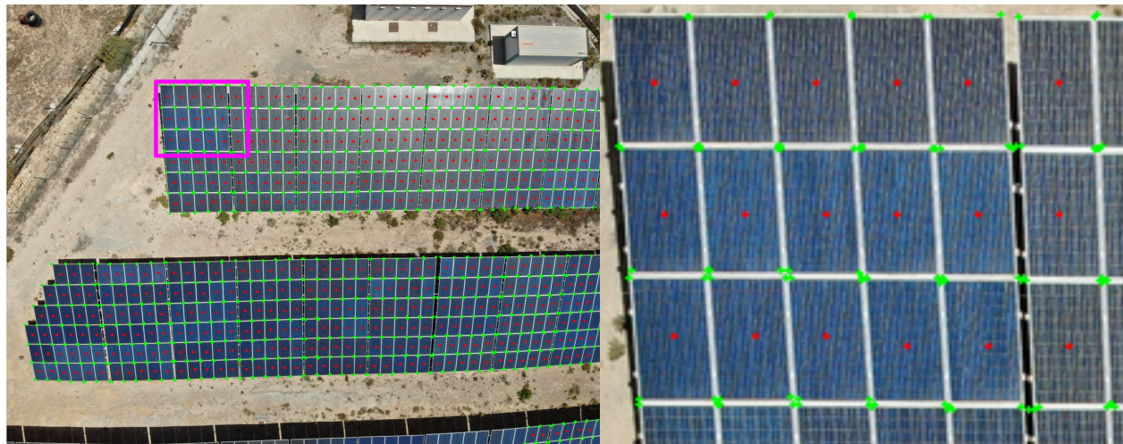
Figure 6.4: Detection results. On the left, full image of 1024x1376 provided to the detector. On the right, a zoom in of the magenta bounding box. Object center detections are depicted with red dots, while the green dots depicts the detected keypoints per object.
