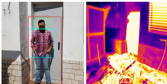
(e) Case 3: Good detection of people in front of heat sources for RGB method (f) Case 3: Bad detection of people in front of heat sources for Thermal method
