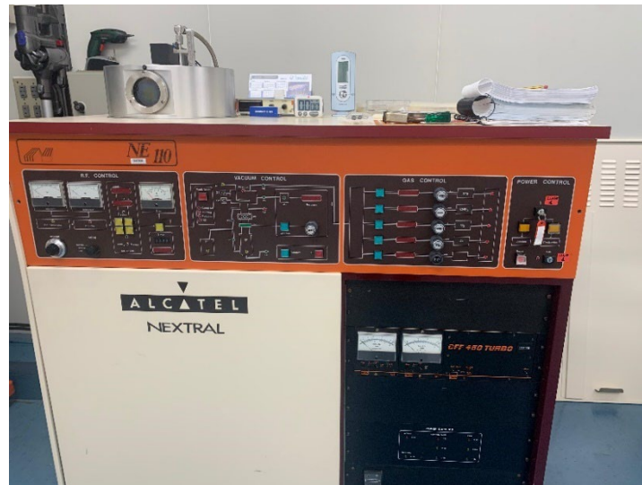
Figure 2.10. Dry Etching system.
