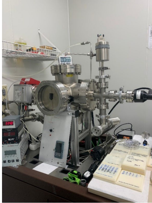
Figure 2.7. Customized CVD tool for CNT growth.
